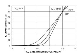
Figure 5. Transfer Characteristics.
