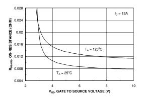
Figure 4. On-Resistance Variation with Gate-to-Source Voltage.
