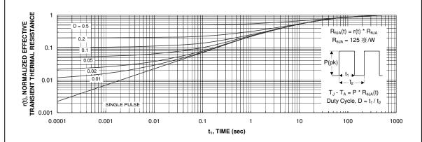
Figure 12. Transient Thermal Response Curve.
