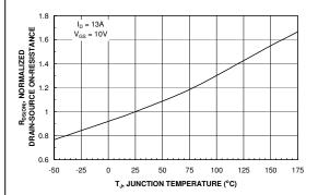
Figure 3. On-Resistance Variation with Temperature.
