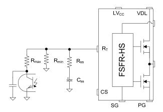
Figure 21. Frequency Control Circuit
