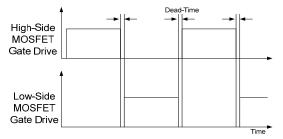
Figure 18. MOSFET Gate Drive Signals
