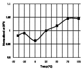
Figure 16. t<sub>DELAY,RESET</sub> vs. Temperature
