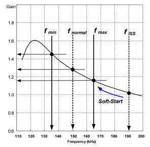
Figure 20. Resonant Converter Typical Gain Curve
