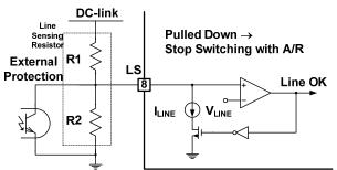
Figure 26. External Protection Circuits
