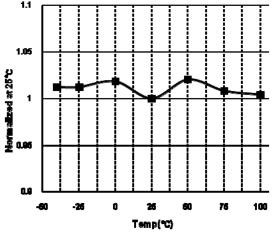
Figure 17. V<sub>RT,RESET</sub> vs. Temperature
