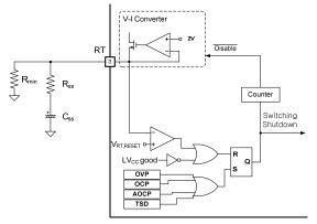
Figure 22. Internal Block for Auto-Restart
