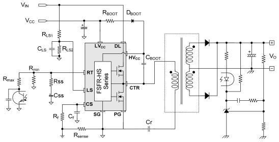
Figure 1. Typical Application Circuit (LLC Resonant Half-Bridge Converter)
