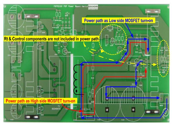
Figure 30. Example of Duty Balancing
