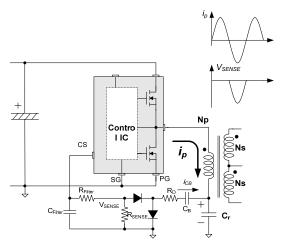
Figure 29. Capacitive Sensing
