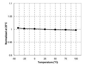
Figure 8. Low-Side  $V_{CC}$  (LV<sub>CC</sub>) Start vs. Temperature
