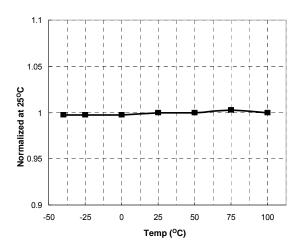
Figure 13. OCP Voltage vs. Temperature
