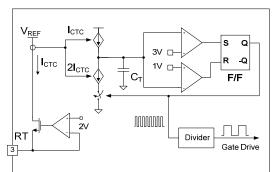
Figure 19. Current-Controlled Oscillator
