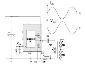
Figure 28. Full-Wave Sensing
