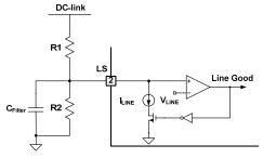
Figure 25. Half-Wave Sensing
