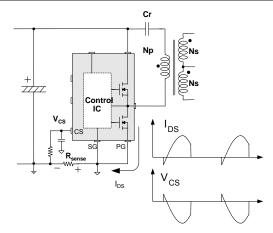
Figure 27. Half-Wave Sensing
