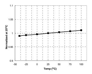
Figure 10. LV<sub>CC</sub> OVP Voltage vs. Temperature
