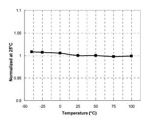
Figure 6. High-Side  $V_{CC}$  (HV<sub>CC</sub>) Start vs. Temperature
