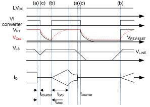
(a) Protection Trigger, (b) FSFR-HS Restart, (c) Counter Stop
