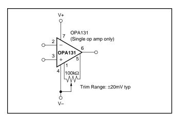
FIGURE 1. OPA131 Offset Voltage Trim Circuit.
