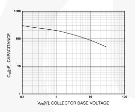
Figure 3. Collector Capacitance
