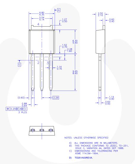
Figure 8. TO-251 (IPAK) MOLDED, 3-LEAD (ACTIVE)
