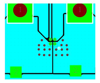
Figure 9. Routing Example 1 oz, 2 Layers, 100°C/W
