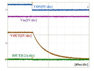
Figure 19. Turn-Off Response – FPF1203 ( $V_{IN}$ =3.3 V,  $C_{IN}$ =1  $\mu F$ ,  $C_{OUT}$ =0.1  $\mu F$ ,  $R_L$ =500  $\Omega$ )
