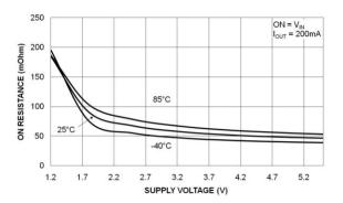
Figure 14. Ron vs. Supply Voltage
