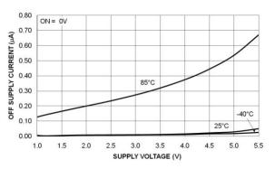
Figure 10. Off Supply Current vs. Supply Voltage  $(V_{\text{OUT}}$  Floating)
