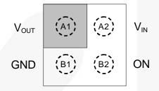
Figure 5. Pin Assignments (Top View)
