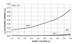
Figure 8. Shutdown Current vs. Supply Voltage
