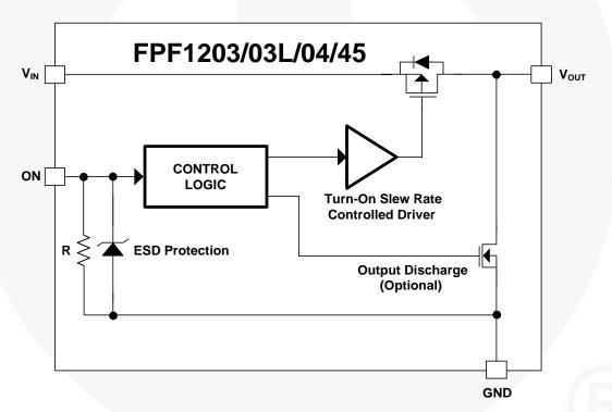
Figure 2. Functional Block Diagram (Output Discharge for FPF1204 / 45)
