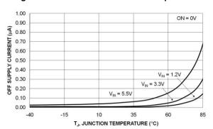
Figure 9. Off Supply Current vs. Temperature (V<sub>OUT</sub> Floating)
