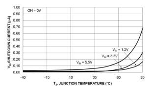
Figure 7. Shutdown Current vs. Temperature
