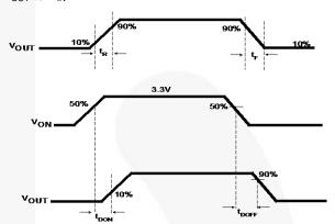
Figure 23. Timing Diagram for FPF1203/4/045
