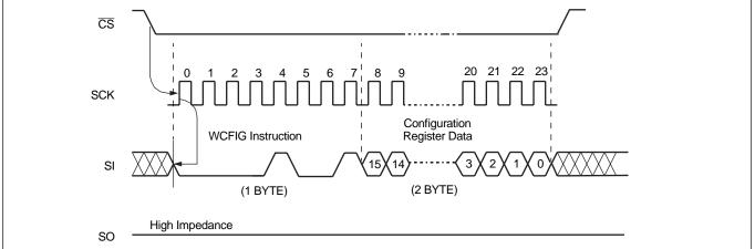
Figure 17. Write Control Register (WCNTR) Operation Sequence
