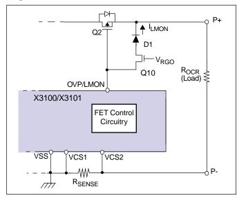
The 5VDC voltage regulator output (V<sub>RGO</sub>) is always active during an over-current protection mode.
