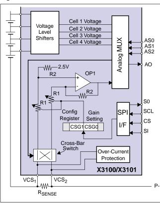
The internal gain of the X3100 or X3101 current sense voltage amplifier can be selected by using the WCNTR Instruction to set bits CSG1 and CSG0 in the control register (Table 14). The CSG1 and CSG0 bits select one of four input resistors to Op Amp OP1. The feedback resistors remain constant. This ratio of input to feedback resistors determines the gain. Putting external resistors in series with the inputs reduces the gain of the amplifier.
