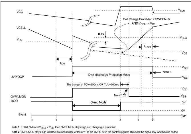
Figure 6. Over-discharge Protection Mode—Event Diagram
