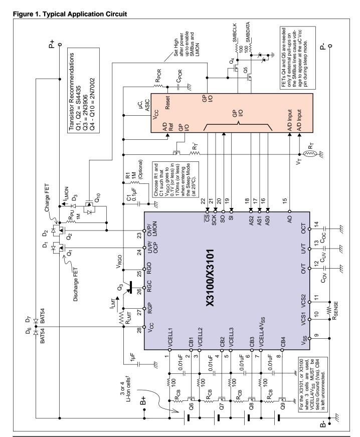
OVP/LMON will be (at maximum) equal to the voltage of the battery terminal, minus one forward biased diode voltage drop ( $V_{P+}$ – $V_{D7}$ ). Since the drain of Q2 is connected to a higher potential ( $V_{P+}$ ) a pull-up resistor ( $R_{PU}$ ) in the order of 1M $\Omega$  should be used to ensure that the charge FET is completely turned OFF when OVP/LMON= $V_{CC}$ .
