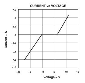
NOTE A: Typical current versus voltage curve was derived using the IEC 1.2/50-μs surge waveform.
