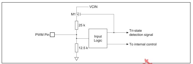
Figure 3 Equivalent Circuit for the PWM-pin Input
