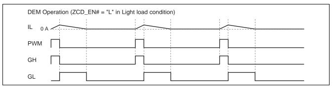
Figure 1.2 Typical Signals during DEM
