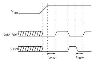
Figure 3. . DATA\_RDY, SHDN Operation Logic Diagram
