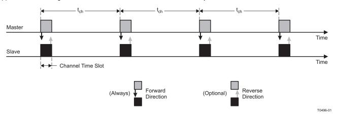
Figure 4. ANT Channel Timing
