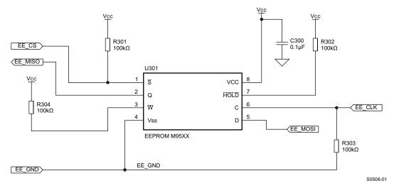
Figure 19. EEPROM Hardware Setup
