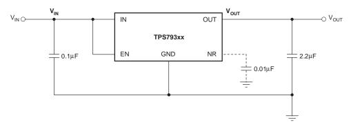
Figure 22. Typical Application Circuit
