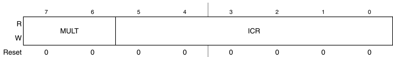
Figure 11-4. IIC Frequency Divider Register (IICF)
