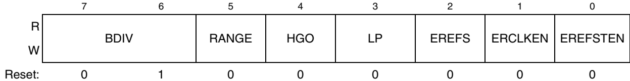
Figure 8-4. ICS Control Register 2 (ICSC2)
