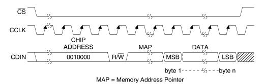
Figure 11. Control Port Timing, SPI mode
