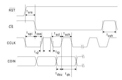
Figure 2. Control Port Timing - SPI Mode
