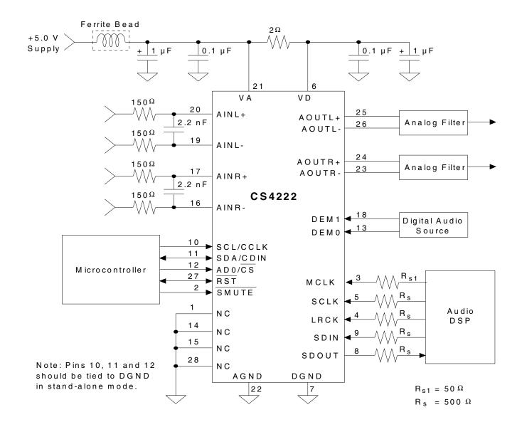
Figure 4. CS4222 Recommended Connection Diagram
