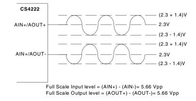
Figure 6. Full Scale Input/Output Voltage
