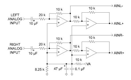
Figure 5. Optional Line Input Buffer
