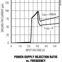
**GROUND-PIN CURRENT vs. INPUT VOLTAGE**
