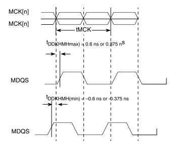
Figure 4. Timing Diagram for tDDKHMH
