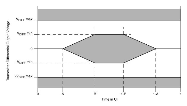
Figure 58. Transmitter Output Compliance Mask
