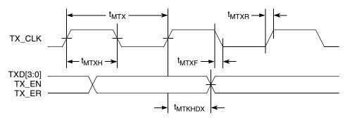
Figure 12. MII Transmit AC Timing Diagram
