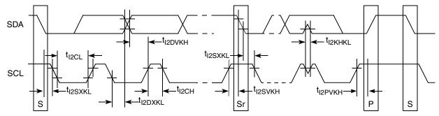
Figure 41. I<sup>2</sup>C Bus AC Timing Diagram
