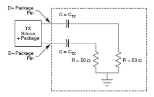
Figure 57. Compliance Test/Measurement Load
