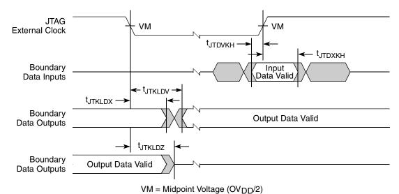
Figure 39. Boundary-Scan Timing Diagram
