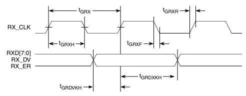
Figure 11. GMII Receive AC Timing Diagram
