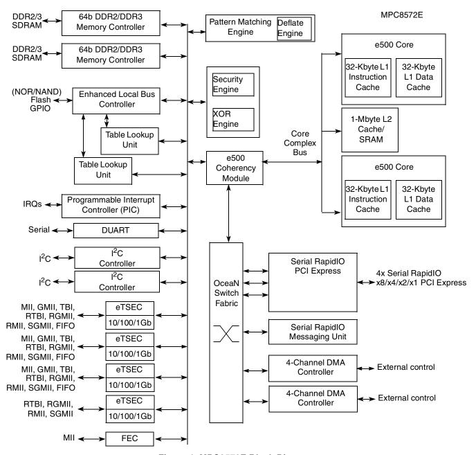
Figure 1. MPC8572E Block Diagram
