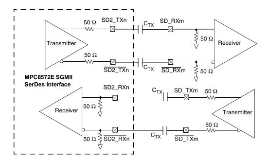
Figure 22. 4-Wire AC-Coupled SGMII Serial Link Connection Example
