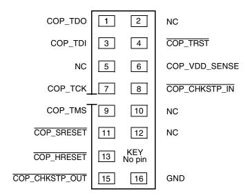
Figure 65. COP Connector Physical Pinout
