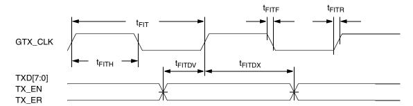
Figure 7. FIFO Transmit AC Timing Diagram
