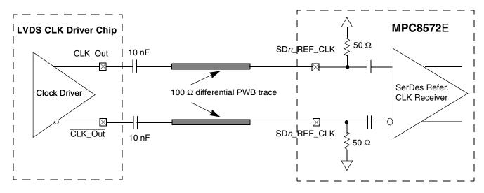
Figure 49. AC-Coupled Differential Connection with LVDS Clock Driver (Reference Only)
