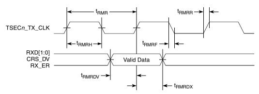
Figure 21. RMII Receive AC Timing Diagram
