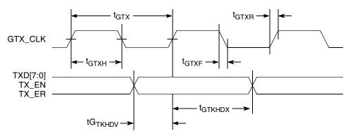
Figure 9. GMII Transmit AC Timing Diagram
