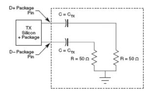
Figure 25. SGMII AC Test/Measurement Load
