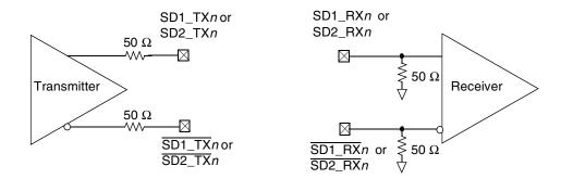
Figure 54. SerDes Transmitter and Receiver Reference Circuits
