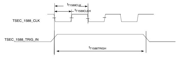
Figure 27. eTSEC IEEE 1588 Input AC timing
