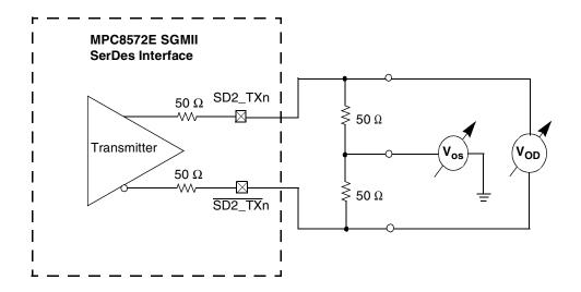
Figure 23. SGMII Transmitter DC Measurement Circuit
