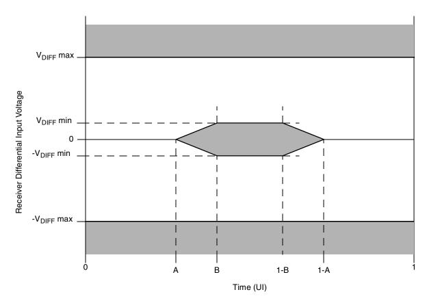
Figure 60. Receiver Input Compliance Mask
