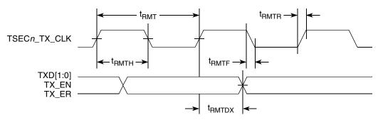
Figure 19. RMII Transmit AC Timing Diagram
