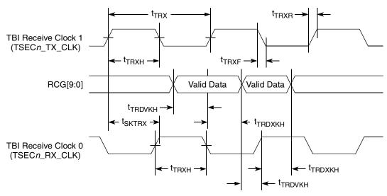
Figure 16. TBI Receive AC Timing Diagram
