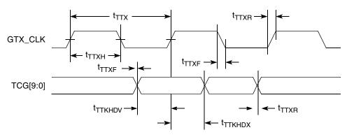
Figure 15. TBI Transmit AC Timing Diagram
