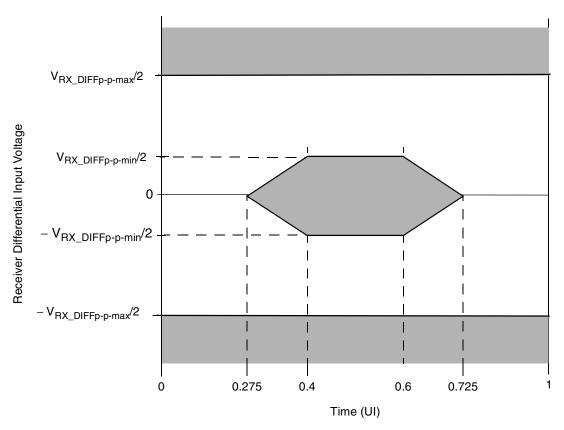
Figure 24. SGMII Receiver Input Compliance Mask
