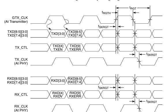
Figure 18 shows the RGMII and RTBI AC timing and multiplexing diagrams.
