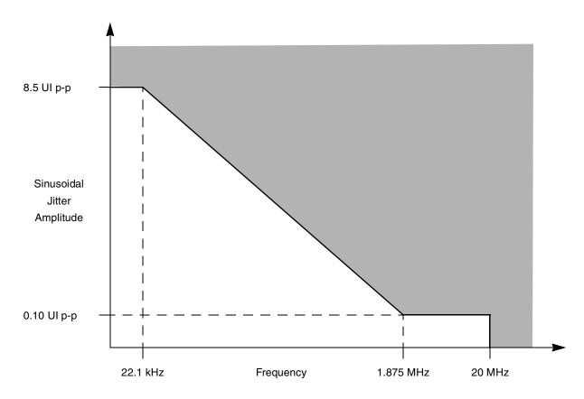
Figure 59. Single Frequency Sinusoidal Jitter Limits
