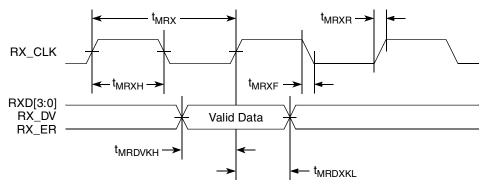
Figure 14. MII Receive AC Timing Diagram
