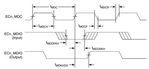
Figure 28. MII Management Interface Timing Diagram
