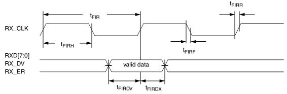
Figure 8. FIFO Receive AC Timing Diagram
