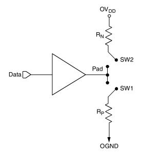
Figure 64. Driver Impedance Measurement
