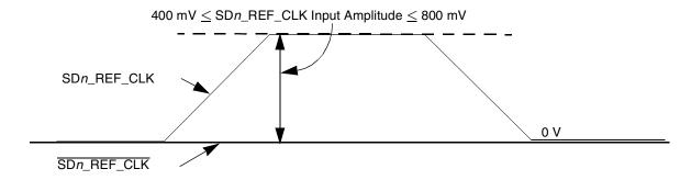
Figure 47. Single-Ended Reference Clock Input DC Requirements
