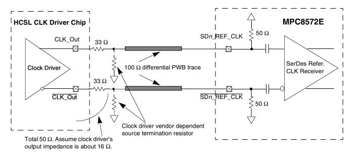
Figure 48. DC-Coupled Differential Connection with HCSL Clock Driver (Reference Only)
