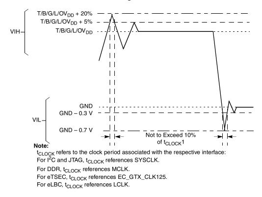
Figure 2. Overshoot/Undershoot Voltage for  $TV_{DD}/BV_{DD}/GV_{DD}/LV_{DD}/OV_{DD}$
