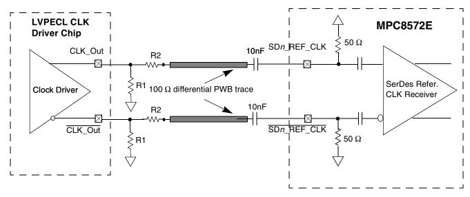
Figure 50. AC-Coupled Differential Connection with LVPECL Clock Driver (Reference Only)
