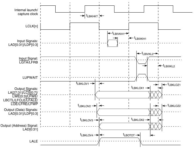
Figure 31. Local Bus Signals (PLL Bypass Mode)
