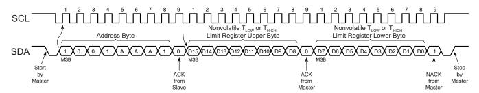
Note: Assumes the Pointer Register was previously set to point to the Nonvolatile  $T_{LOW}$  or  $T_{HIGH}$  Limit Register.
