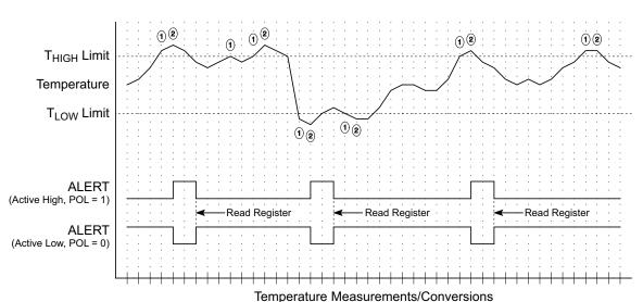
Figure 5-3. Interrupt Mode (Fault Tolerance Queue = 2)
