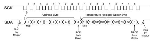
Note: Assumes the Pointer Register was previously set to point to the Temperature Register.
