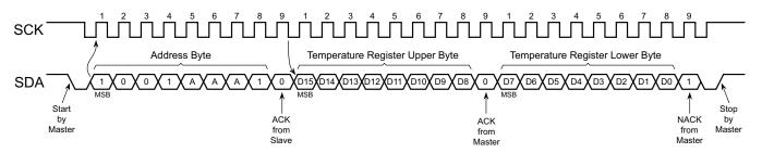
Note: Assumes the Pointer Register was previously set to point to the Temperature Register.
