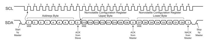
Note: Assumes the Pointer Register was previously set to point to the Nonvolatile Configuration Register.
