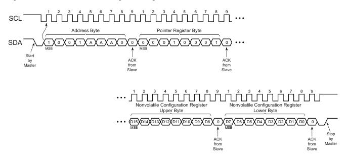
Figure 6-7. Read from Nonvolatile Configuration Register
