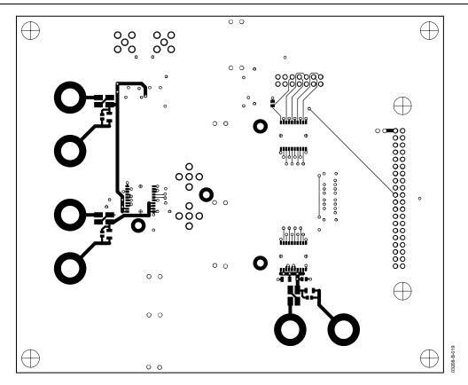
Figure 22. Evaluation Board Top Layer Copper
