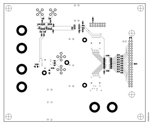
Figure 25. Evaluation Board Bottom Layer Copper
