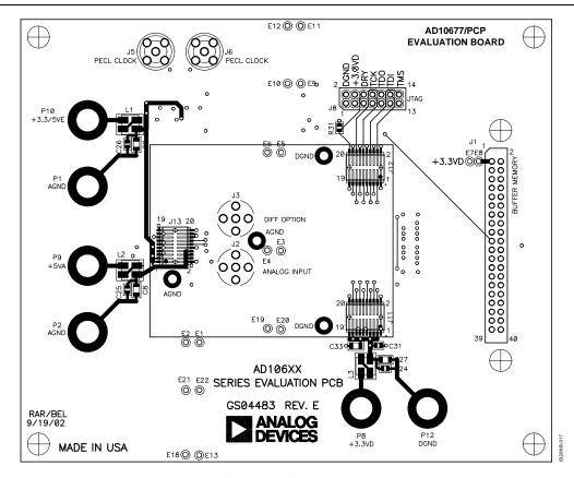
Figure 20. Evaluation Board Mechanical Layout, Top View
