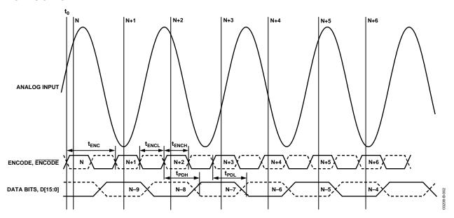
Figure 2. Timing Diagram
