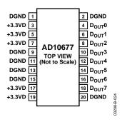
Figure 7. Pin Configuration P2 (See Figure 9)
