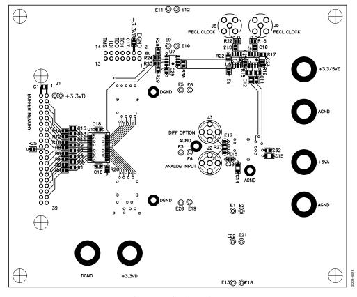
Figure 21. Evaluation Board Mechanical Layout, Bottom View
