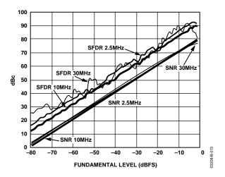
Figure 16. SFDR and SNR vs. Analog Input Level
