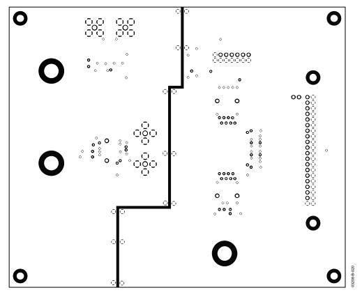
Figure 23. Evaluation Board Second Layer Copper
