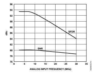
Figure 17. SFDR and SNR vs. Analog Input Frequency
