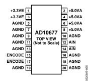
Figure 8. Pin Configuration P3 (See Figure 9)
