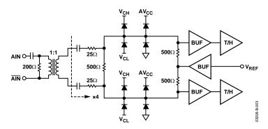
Figure 3. Analog Input Stage
