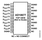
Figure 6. Pin Configuration P1 (See Figure 9)
