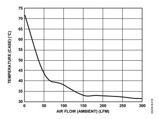
Figure 18. Temperature (Case) vs. Air Flow (Ambient)
