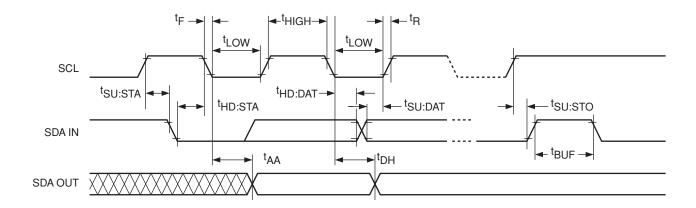
Figure 1. 2-Wire Serial Interface Timing
