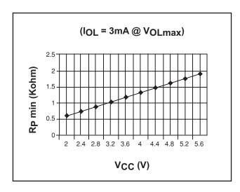
Figure 2. Minimum R<sub>P</sub> Value versus Supply Voltage
