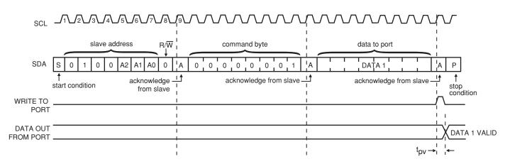
Figure 9. Write to Output Port Register
