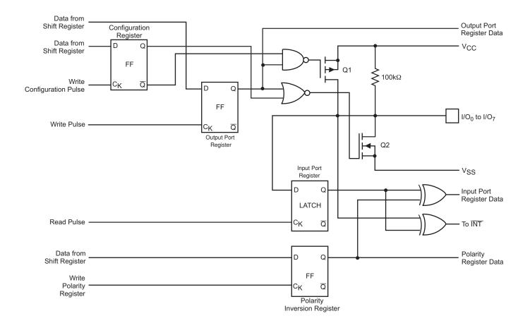
Figure 4. Simplified Schematic of I/O<sub>0</sub> to I/O<sub>7</sub>
