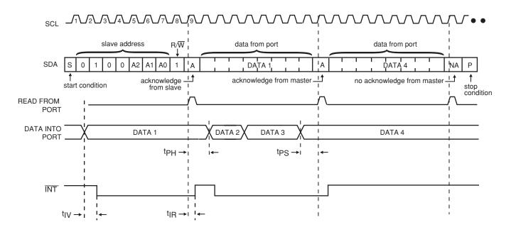
Figure 12. Read Input Port Register
