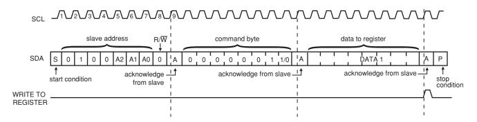
Figure 10. Write to Configuration or Polarity Inversion Register
