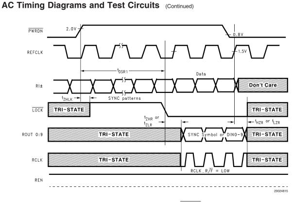
FIGURE 15. Deserializer PLL Lock Times and PWRDN TRI-STATE Delays
