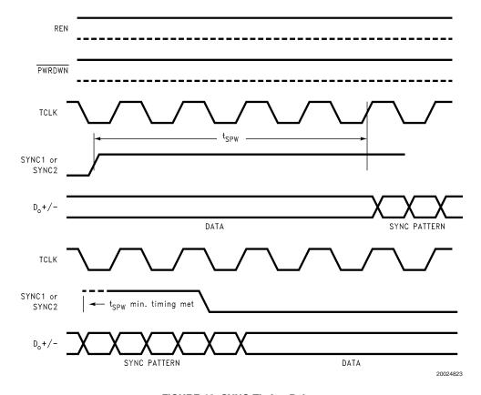
FIGURE 10. SYNC Timing Delays
