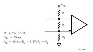
FIGURE 18. Failsafe Biasing Setup
