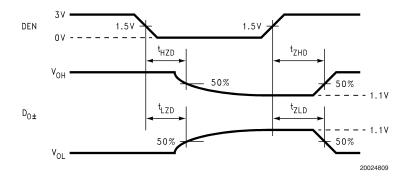
FIGURE 8. Serializer TRI-STATE Test Circuit and Timing
