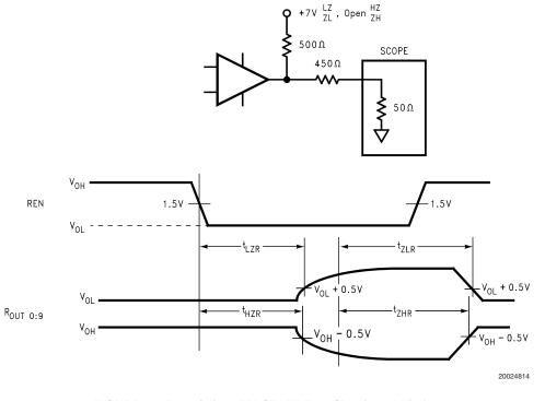
FIGURE 14. Deserializer TRI-STATE Test Circuit and Timing
