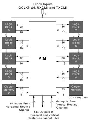
Figure 5. PSI Logic Block Cluster Diagram
