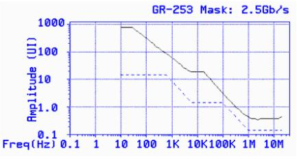
Figure 18. Jitter Tolerance for CYS25G01K100
