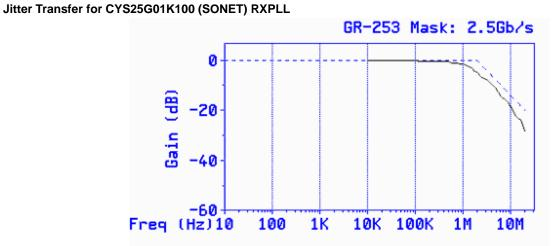
Figure 17. Jitter Transfer for CYS25G01K100
