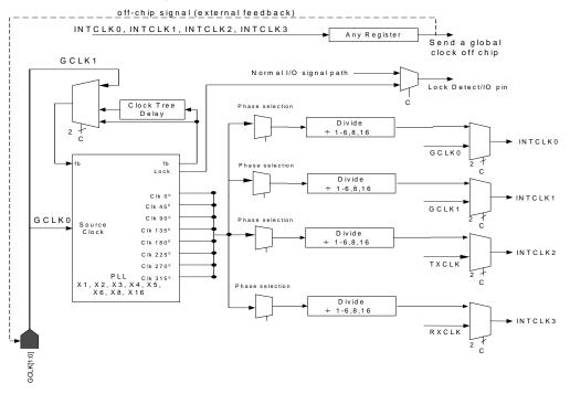
Figure 11. Block Diagram of Spread Aware PLL for CYP25G01K100
