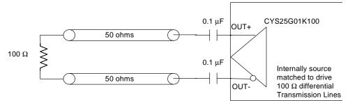
Figure 20. Serial Output Termination
