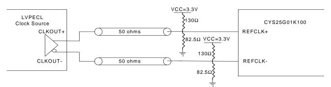
Figure 21. REFCLK Oscillator Termination
