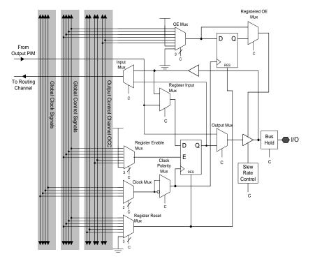
Figure 10. Block Diagram of I/O Cell
