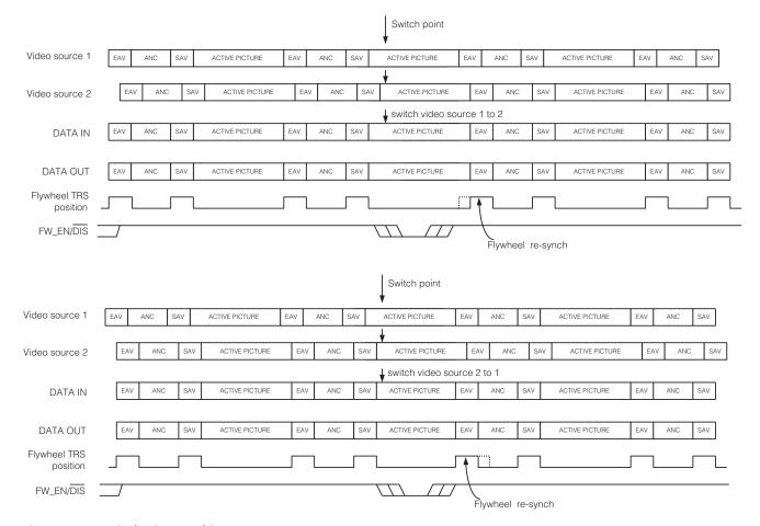
Figure 3-2: Switch Line Locking
