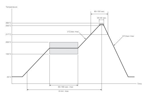
Figure 2-2: Maximum Pb-free Solder Reflow Profile (Pb-free package)
