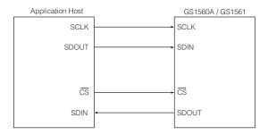
Figure 3-9: Gennum Serial Peripheral Interface (GSPI)
