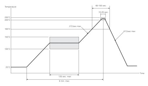
Figure 2-1: Standard Eutectic Solder Reflow Profile
