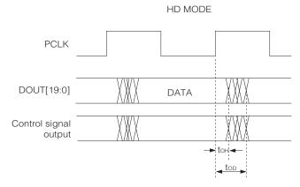
Figure 3-7: HD PCLK to Data Timing
