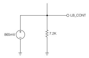
Figure 2-5: PLL Loop Bandwidth Control
