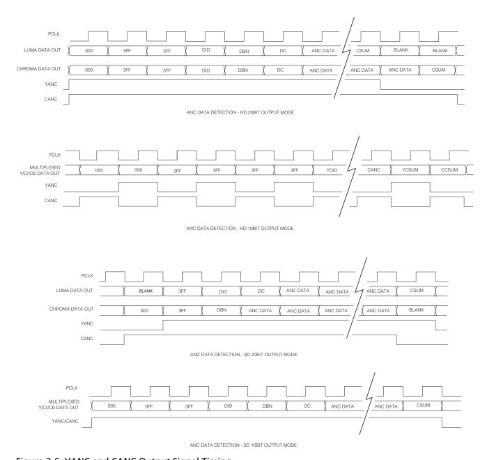
Figure 3-6: YANC and CANC Output Signal Timing
