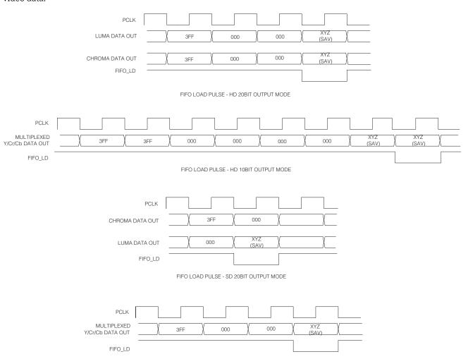
Figure 3-5: FIFO\_LD Pulse Timing
