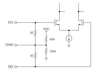
Figure 2-3: Serial Digital Input
