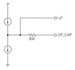
Figure 2-7: VCO Control Output & PLL Lock Time Capacitor
