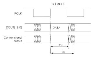
Figure 3-8: SD PCLK to Data Timing
