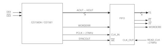
Figure 3-4: DVB-ASI FIFO Implementation Using The GS1560A
