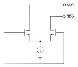
Figure 2-6: Serial Digital Output (GS1560A only)
