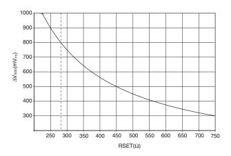
Figure 3-1: Serial Digital Loop-Through Output Swing
