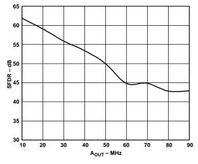
Figure 4. Wideband SFDR (200 MHz Clock) vs.  $A_{OUT}$
