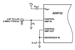
Figure 18. Lower Frequency Multiplying Circuit
