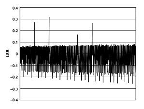
Figure 7. Typical Differential Nonlinearity Performance (DNL)
