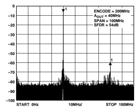
Figure 13. Wideband SFDR 40 MHz A<sub>OUT</sub>; 200 MHz Clock
