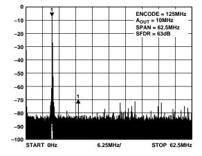
Figure 10. Wideband SFDR 10 MHz  $A_{OUT}$ ; 125 MHz Clock
