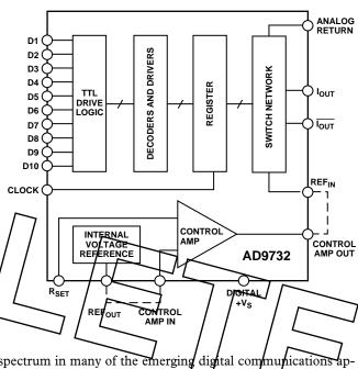
spectrum in many of the emerging digital communications applications where signal purity is critical. Narrowband (±1 MHz window), the AD9732 provides an SFDR of greater than 75 dB. This level of wideband and narrowband ac performance, coupled with its 200 MSPS throughput rate, enables the AD9732 to present outstanding value in the high speed DAC function.
