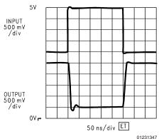
LM7131 Driving Flash A/D Load  $A_V = +1$  @ +5V
