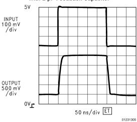
LM7131 Driving Flash A/D Load  $A_V = +10 @ +5V$
