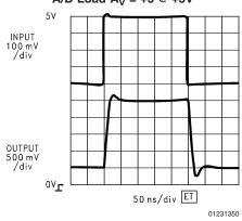
LM7131 Driving Flash A/D Load A<sub>V</sub> = +5 @ +5V With 2 pF Feedback Capacitor
