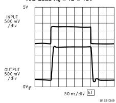
LM7131 Driving Flash A/D Load  $A_V = +5$  @ +5V
