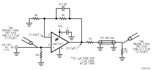
Numbers in parentheses are measured fixture capacitances w/o DUT and load.
