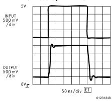
LM7131 Driving Flash A/D Load A<sub>V</sub> = +2 @ +5V
