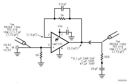
Numbers in parentheses are measured fixture capacitances w/o DUT and load.
