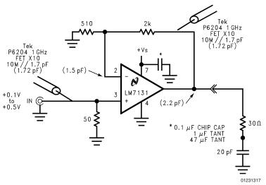
Numbers in parentheses are measured fixture capacitances w/o DUT and load.
