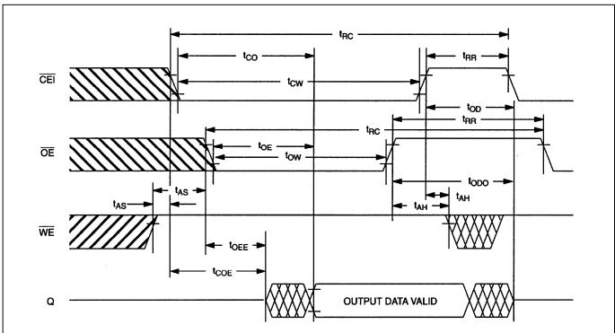
Figure 8. Timing Diagram: Read Cycle to Time Chip ROM/ $\overline{RAM} = V_{CCO}$
