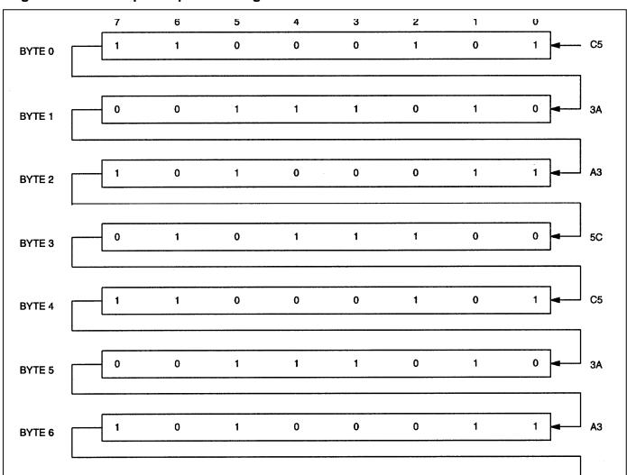
Figure 2. Time Chip Comparison Register Definition
