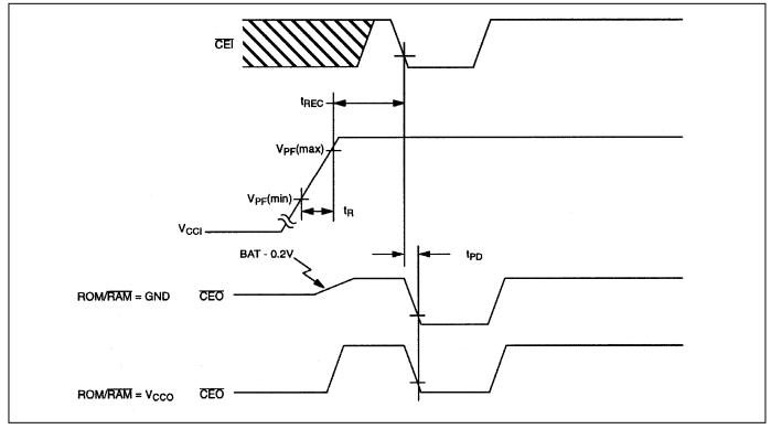
Figure 12. 5V Power-Down Condition
