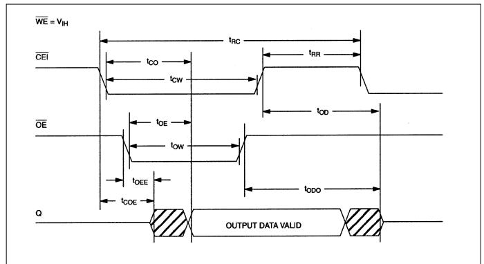
Figure 6. Timing Diagram: Read Cycle to Time Chip ROM/ $\overline{RAM}$  = GND
