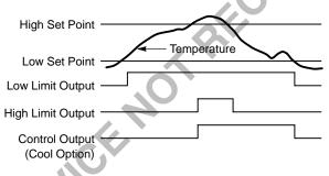
Figure 2. MC623 Temperature vs. Output
