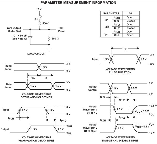
NOTE A: CL includes probe and jig capacitance.
