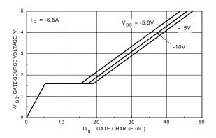
Figure 10. Gate Charge Characteristics.
