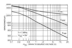
Figure 9. Capacitance Characteristics.
