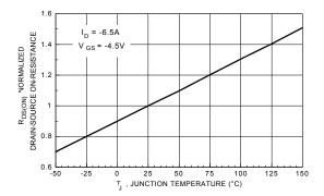
Figure 3. On-Resistance Variation with Temperature.
