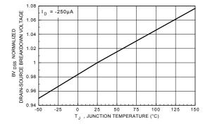
Figure 7. Breakdown Voltage Variation with Temperature.
