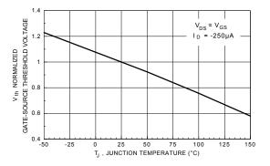
Figure 6. Gate Threshold Variation with Temperature.
