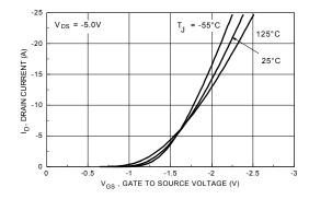
Figure 5. Transfer Characteristics.
