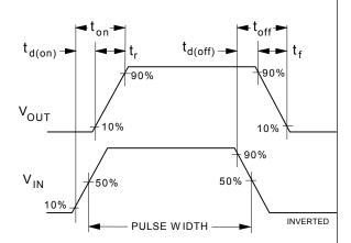
Figure 12. Switching Waveforms.
