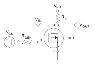
Figure 11. Switching Test Circuit.
