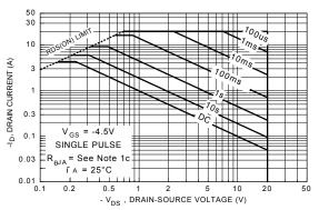
Figure 15. Maximum Steady-State Drain
