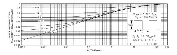
Figure 17. Transient Thermal Response Curve.
