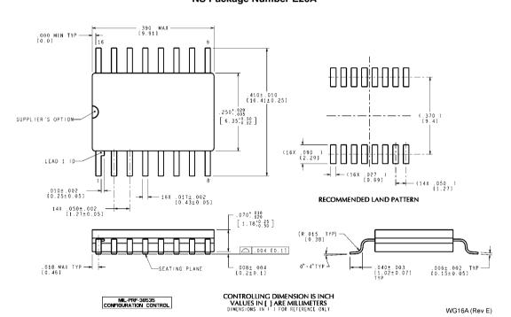
Ceramic SOIC NS Package Number WG16A
