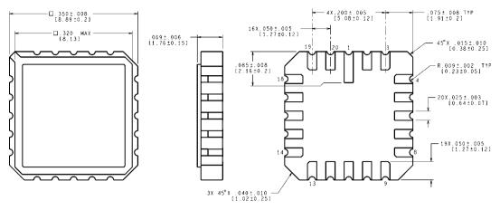
CONTROLLING DIMENSION IS INCH VALUES IN [] ARE MILLIMETERS
