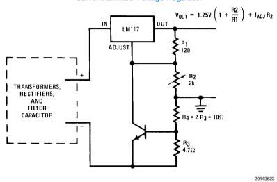
– Short circuit current is approximately  $\frac{600 \text{ mV}}{\text{R3}}$ , or 120 mA
