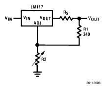
FIGURE 2. Regulator with Line Resistance in Output Lead
