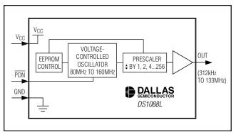
Figure 1. Block Diagram
