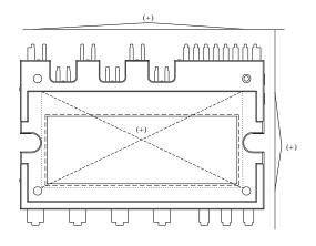
Figure 6. Flatness Measurement Position
