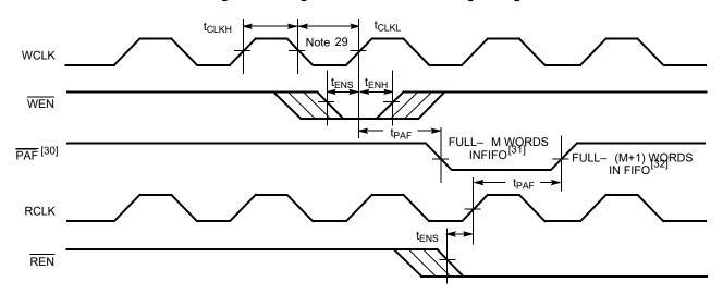
Figure 16. Programmable Almost Full Flag Timing (applies only in SMODE (SMODE is LOW))
