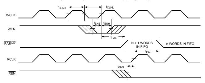
Figure 14. Programmable Almost Empty Flag Timing (applies only in SMODE (SMODE is LOW))
