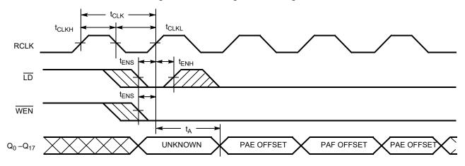
Figure 19. Write Expansion Out Timing
