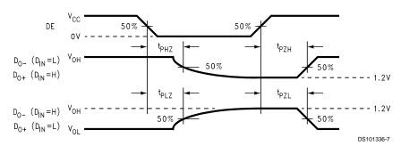
FIGURE 5. Driver TRI-STATE Delay Waveforms
