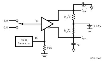
FIGURE 4. Driver TRI-STATE Delay Test Circuit
