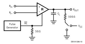
FIGURE 8. Receiver TRI-STATE Delay Test Circuit
