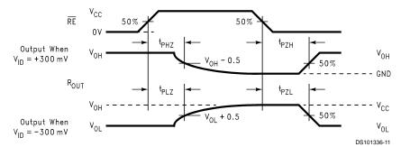
FIGURE 9. Receiver TRI-STATE Delay Waveforms
