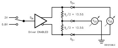
FIGURE 1. Differential Driver DC Test Circuit
