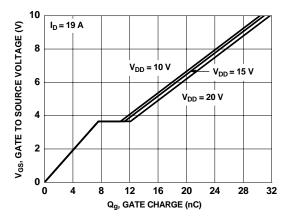
Figure 7. Gate Charge Characteristics
