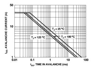
Figure 9. Unclamped Inductive Switching Capability
