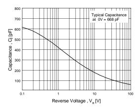
Figure 3. Typical Junction Capacitance
