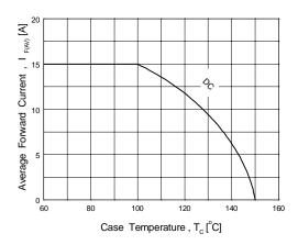
Figure 6. Forward Current Derating Curve
