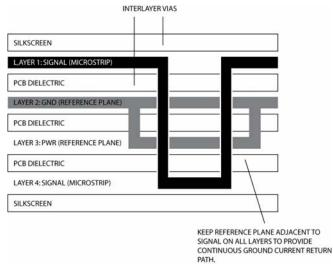
Figure 32. Example Routing of Reference Plane
