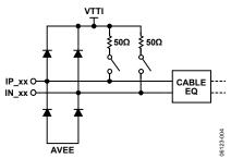
Figure 25. High Speed Input Simplified Schematic
