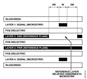
Figure 33. Example Board Stackup
