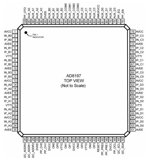
Figure 3. Pin Configuration
