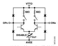
Figure 26. High Speed Output Simplified Schematic
