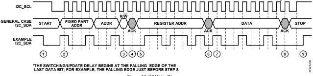
Figure 29. I<sup>2</sup>C Write Diagram
