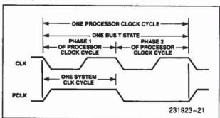
Figure 21. System and Processor Clock Relationships
