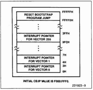
Figure 9. 8086 Real Address Mode Initially Reserved Memory Locations
