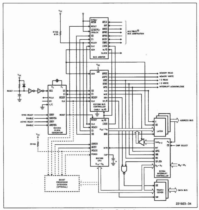
Figure 33. MULTIBUS System Bus Interface
