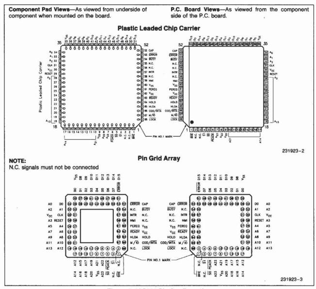
Figure 2. 80C286 Pin Configuration
