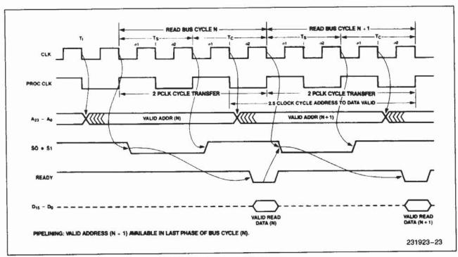
Figure 23. Basic Bus Cycle
