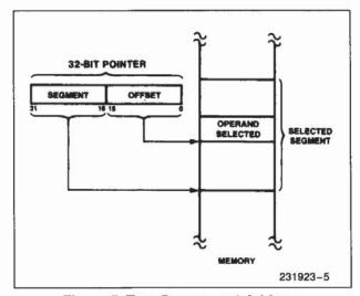
Figure 5. Two Component Address
