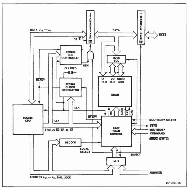
Figure 34. 80C286 System Configuration with Dual-Ported Memory
