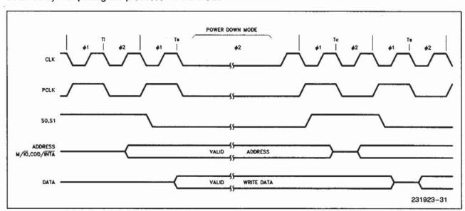
Figure 31. Example Power-Down Sequence
