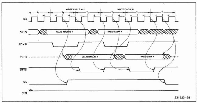
Figure 28. Back to Back Write-Write Cycles
