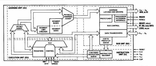
Figure 1. 80C286 Internal Block Diagram
