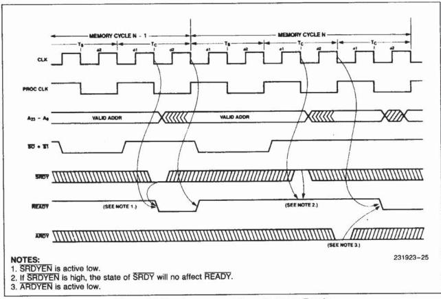
Figure 25. Synchronous and Asynchronous Ready
