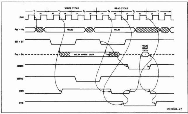
Figure 27. Back to Back Write-Read Cycles
