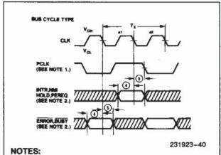
PCLK indicates which processor cycle phase will occur on the next CLK. PCLK may not indicate the correct phase until the first bus cycle is performed.
