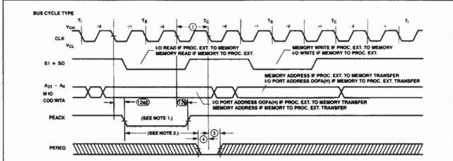
ASSUMING WORD-ALIGNED MEMORY OPERAND, IF ODD ALIGNED, 80286 TRANSPERS TO/FROM MEMORY SYTE-AT-A-TIME WITH TWO MEMORY CYCLES.
