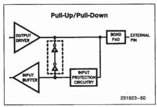
Figure Ba. Bus Hold Circuitry Pins 36-51, 66-67
