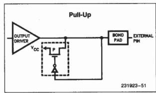
Figure Bb. Bus Hold Circuitry Pins 4-6, 68
