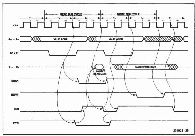
Figure 26. Back to Back Read-Write Cycles
