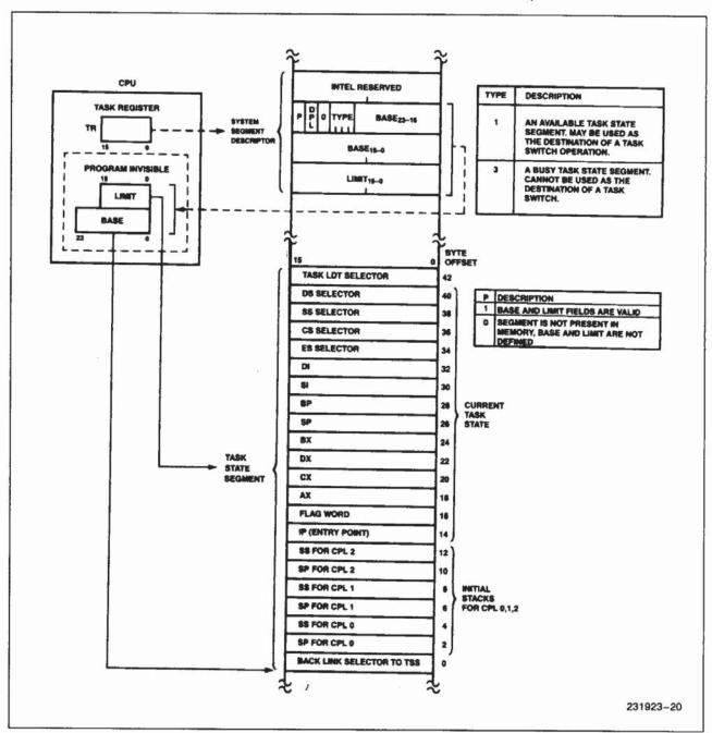
Figure 20. Task State Segment and TSS Registers
