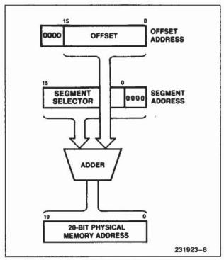
Figure 8. 8086 Real Address Mode Address Calculation
