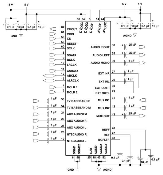
Figure 4–2. Application Schematic
