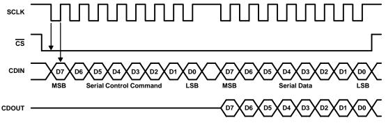
Figure 2–5. Serial Interface Timing
