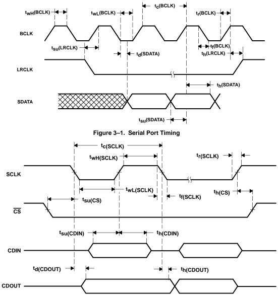
Figure 3–2. SPI Serial Control Port Timing
