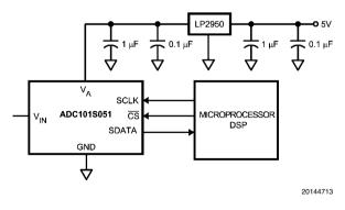
FIGURE 6. Typical Application Circuit
