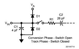
FIGURE 7. Equivalent Input Circuit
