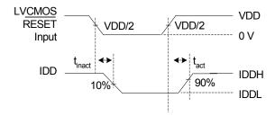
Figure 2. Voltage Waveforms Enable and Disable Times Low- and High-level Enabling<sup>[11]</sup>
