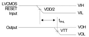
Figure 4. Voltage Waveforms Propagation Delay Times<sup>[11]</sup>
