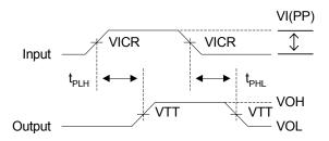
Figure 3. Voltage Waveforms Propagation Delay Times<sup>[12]</sup>
