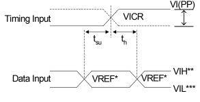
Figure 1. Voltage Waveforms Set-up and Hold Times<sup>[11, 13, 14]</sup>
