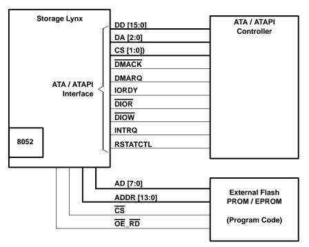
Figure 2–4. Mode 1, ATA/ATAPI Bridge, External ROM
