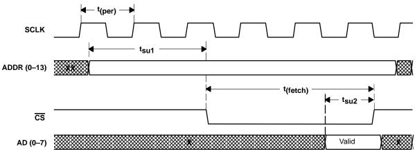
Figure 7–1. External Flash Instruction Fetch Timing
