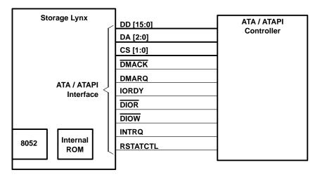
Figure 2–3. Mode 0, ATA/ATAPI Bridge, Internal ROM
