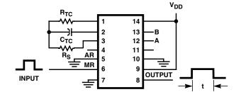
FIGURE 3. DIGITAL TIMER APPLICATION CIRCUIT
