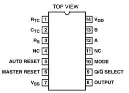
The output from this timer is the Q or  $\overline{Q}$  output from the 8th, 10th, 13th, or 16th counter stage. The desired stage is chosen using time-select inputs A and B (see Frequency Select Table).
