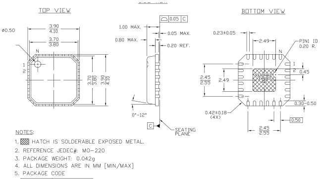
Figure 11. 24-Pin QFN 4 × 4 mm (Subcon Punch Type Pkg with 2.49 × 2.49 EPAD) LF24A/LY24A
