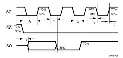
FIGURE 2. Data Output Timing Diagram
