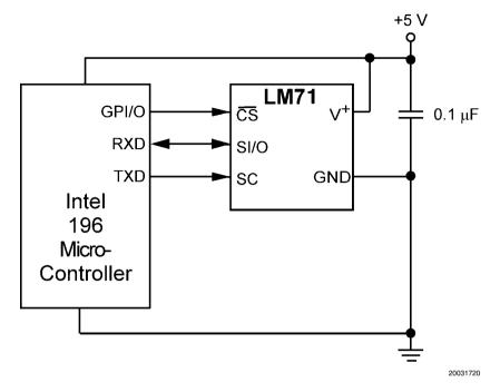
FIGURE 8. Temperature monitor using Intel 196 processor
