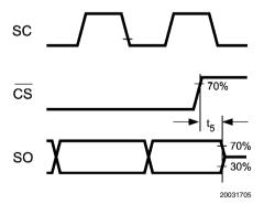
FIGURE 3. TRI-STATE Data Output Timing Diagram
