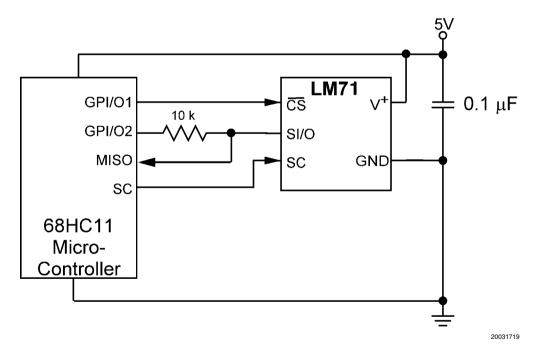
FIGURE 9. LM71 digital input control using micro-controller's general purpose I/O.
