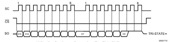
b) Reading Continuous Conversion - Two Eight-Bit Frames
