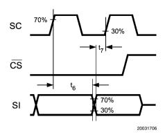
FIGURE 4. Data Input Timing Diagram
