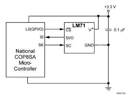
**FIGURE 1. COP Microcontroller Interface**
