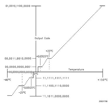
FIGURE 5. Temperature-to-Digital Transfer Function (Non-linear scale for clarity)
