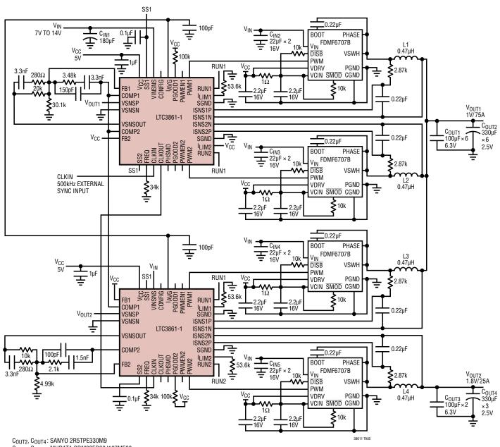
Dual-Output Converter: Triple Phase + Single Phase with DrMOS, Synchronized to an External 500kHz Clock
