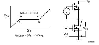
Figure 14. Gate Charge Characteristic
