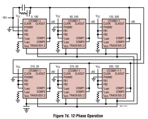
Figure 7. PHSMD Connections for 3-, 4-, 6- or 12-Phase Operation
