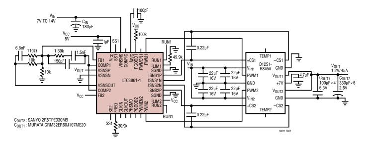
Dual Phase 1.2V/45A Converter with Delta 45A Power Block,  $f_{SW} = 400 kHz$
