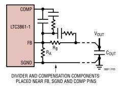
Figure 3. Output Divider and Compensation Component Placement
