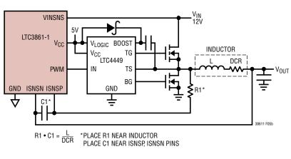
(5b) Using the Inductor to Sense Current
