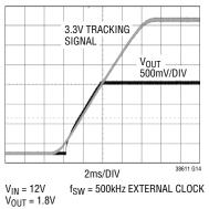
**Ratiometric Tracking (Single** Phase Using FDMF6707B DrMOS)
