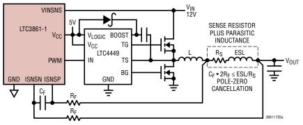
FILTER COMPONENTS PLACED NEAR SENSE PINS
