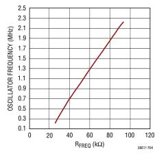
Figure 4. Oscillator Frequency vs R<sub>FREQ</sub>
