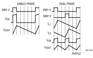
Figure 8. Single and 2-Phase Current Waveforms
