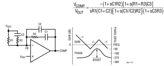
Figure 13. Type 3 Amplifier Compensation
