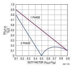
Figure 9. Normalized Output Ripple Current vs Duty Factor  $[I_{RMS}{}^{\prime\prime}$  0.3  $(DI_{C(PP)})]$
