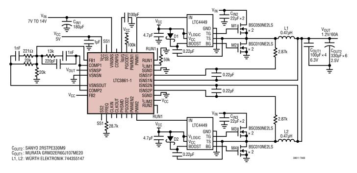
Dual Phase 1.2V/60A Converter with Discrete Gate Drivers and MOSFETs,  $f_{SW}$  = 300kHz
