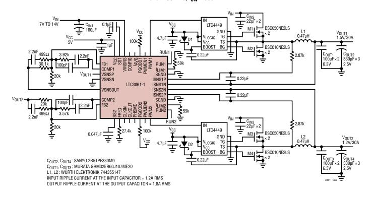
1.5V/30A and 1.2V/30A Converter with Discrete Gate Drivers and MOSFETs,  $f_{SW}$  = 300kHz
