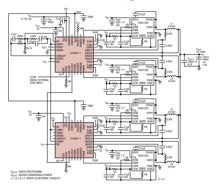
4-Phase 1V/100A Converter with DrMOS, f<sub>SW</sub> = 500kHz
