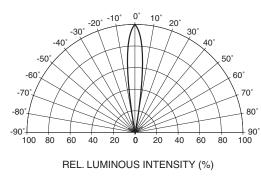
Fig. 4 Radiation Diagram
