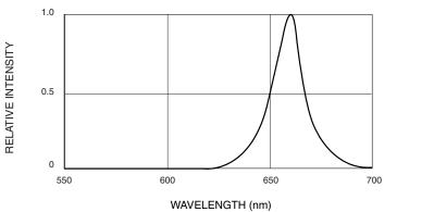
Fig. 3 Relative Intensity vs. Peak Wavelength
