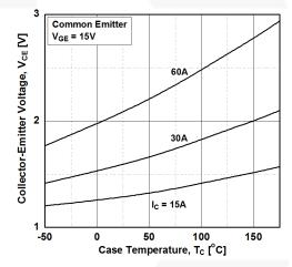
Figure 6. Saturation Voltage vs. V<sub>GE</sub>
