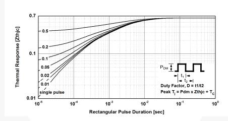
Figure 22. Transient Thermal Impedance of Diode
