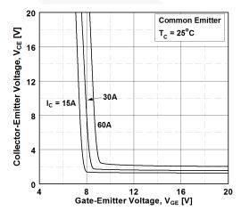
**Figure 2. Typical Output Characteristics**
