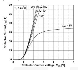
Figure 3. Typical Saturation Voltage Characteristics
