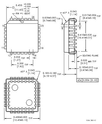
28-Lead Plastic Chip Carrier (PLCC) NS Package Number V28A
