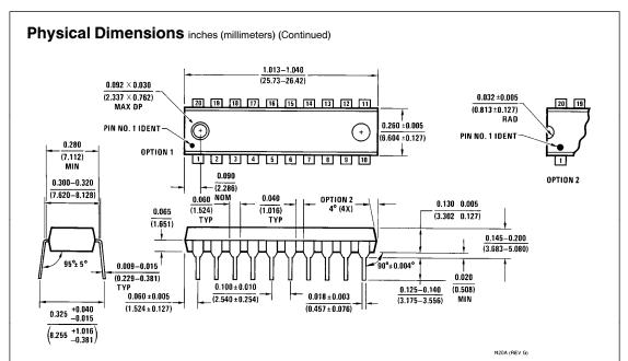
20-Lead Molded Dual-On-Line Package (N) NS Package Number N20A
