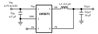
Figure 32. LM3671 Fixed-Voltage Typical Application Circuit
