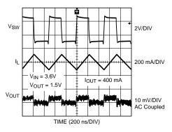
Figure 29. Typical PWM Operation
