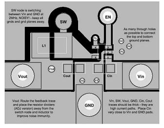
Figure 38. Top Layer Board Layout for SOT-23
