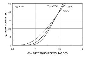
Figure 5. Transfer Characteristics.
