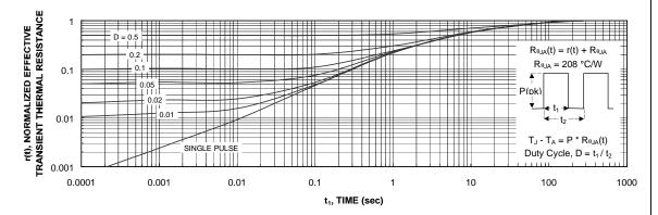
Figure 11. Transient Thermal Response Curve.
