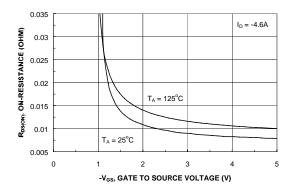
Figure 4. On-Resistance Variation with Gate-to-Source Voltage.
