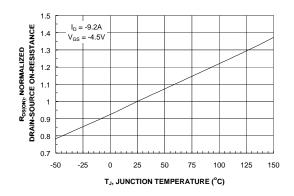
Figure 3. On-Resistance Variation withTemperature.
